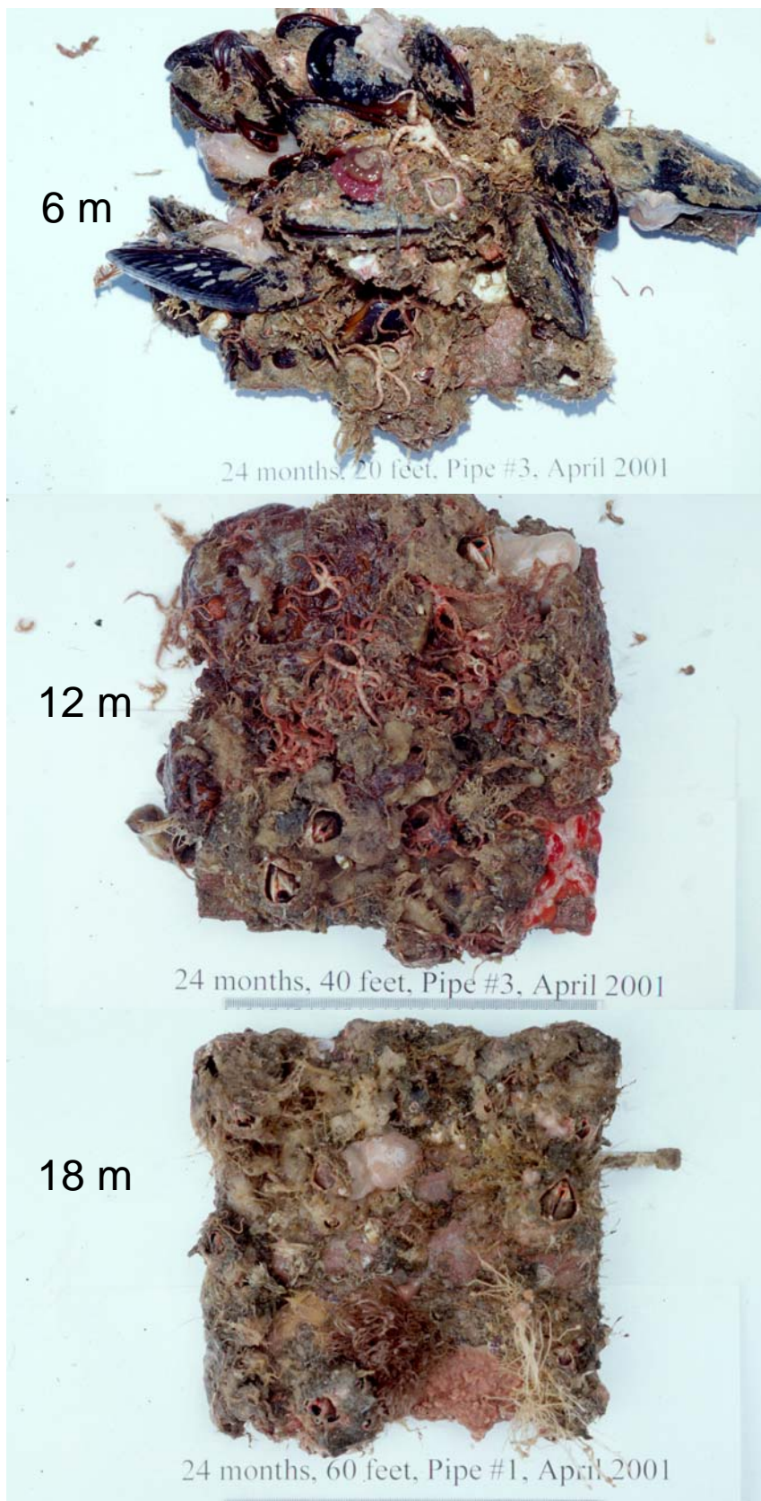
Plate I. Photographs of ceramic tiles submerged for 24 months at depths of 6, 12, and 18 m at Platform Houchin.
