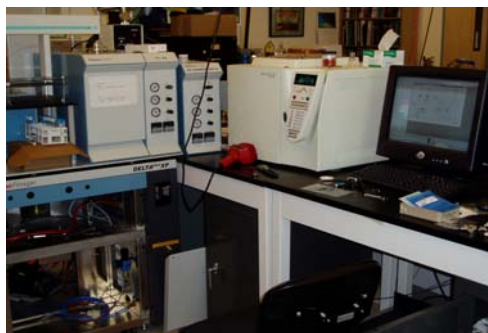
Figure 2. Left panel shows an image of the IR-MS used to determine isotopic values for CO 2 produced during the experiment. Right panel shows initial results for the experimental (E#1), blanks and kill controls during the first 120 days of the experiment.
