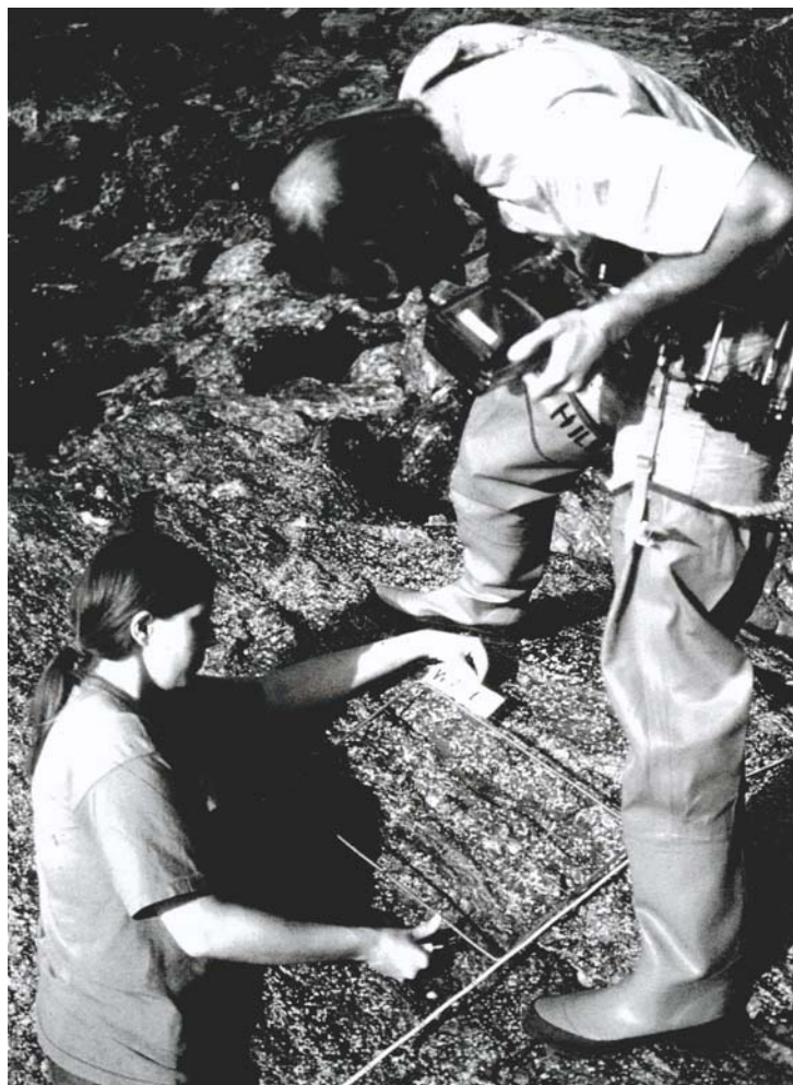
Fig. 6-10. Investigators using a hand-held 35-mm camera equipped with an electronic strobe to photograph the contents of a field plot. The photographer has taken a position directly above the plot so as to photograph its contents at an angle as close as possible to 90° to the plane of the substratum. Usually, a second person is required to provide assistance in positioning and securing plots on shores where topography is heterogeneous and irregular.
