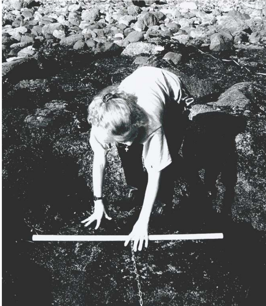
Fig. 5-4. Band transect used for sampling kelp densities. The transect is searched at a prescribed width (e.g., 0.5 m) along each side of the line using a 1.0 m wand.
