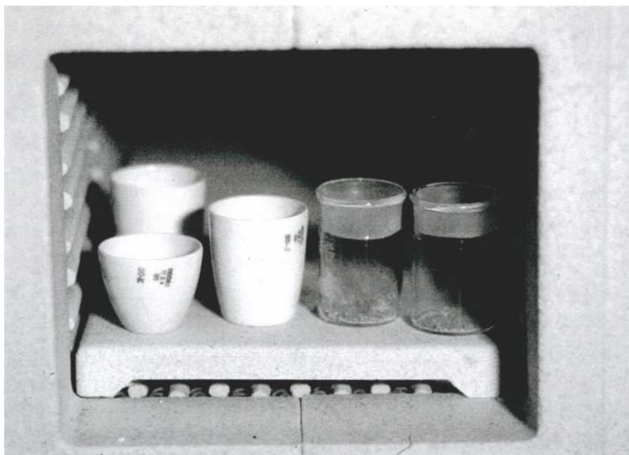
Fig. 7-5. Glass weighing jars and ceramic crucibles containing dried algal powder loaded on the shelf of a muffle furnace prior to ashing.
