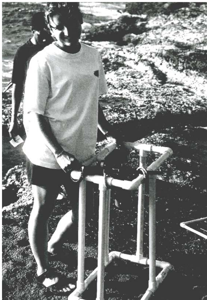
Fig. 6-11. Photographer standing adjacent to a Nikonos camera and an electronic strobe mounted to a fixed stand made of PVC pipe. The base of the stand has been configured to represent the plot borders. All photographs are taken at the same fixed angle and distance with respect to the plot surface.
