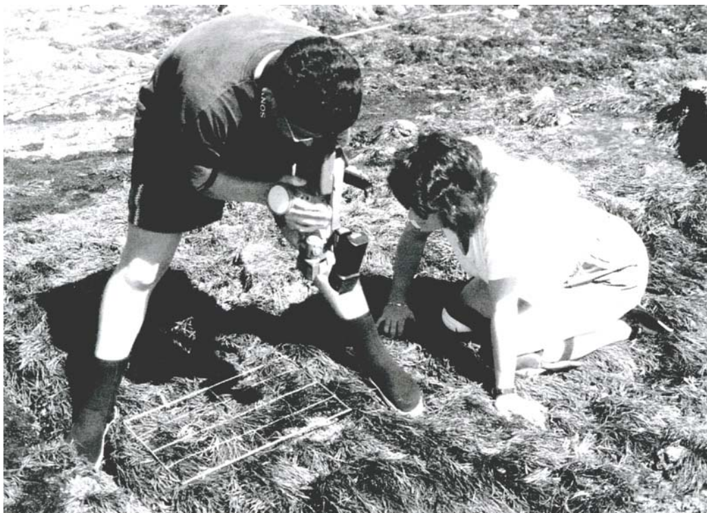
Fig. 6-12. Videographer filming plot contents in the field with a Camcorder equipped with a battery-operated light source. Filming procedures include taking plot views at different scales ranging from full plot photos to macrophotos of small plot sections.
