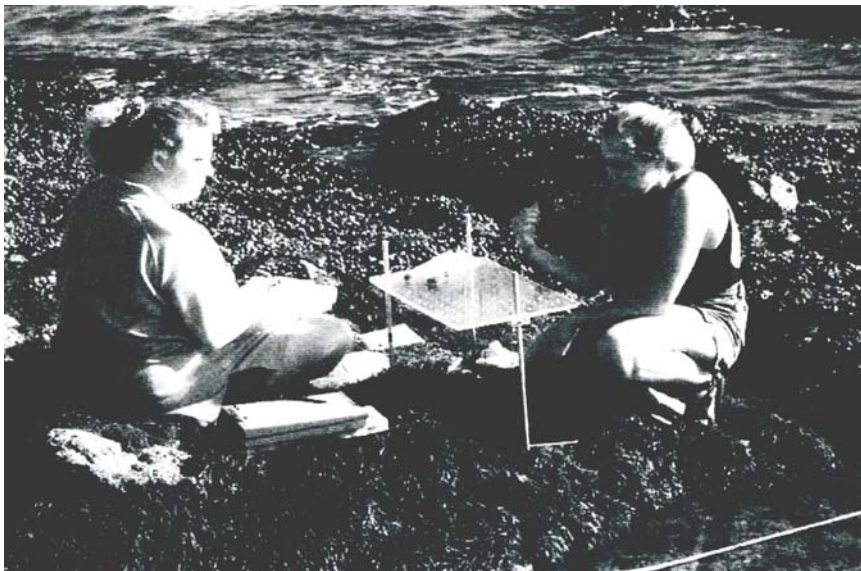
Fig. 2-4. A form of profile gauge for measuring topographic heterogeneity. An array of regularly spaced rods are dropped perpendicularly from the leveled platform and the distance to the substratum is measured. These data can be used to calculate a topographic index using procedures described by Underwood and Chapman (1989).
