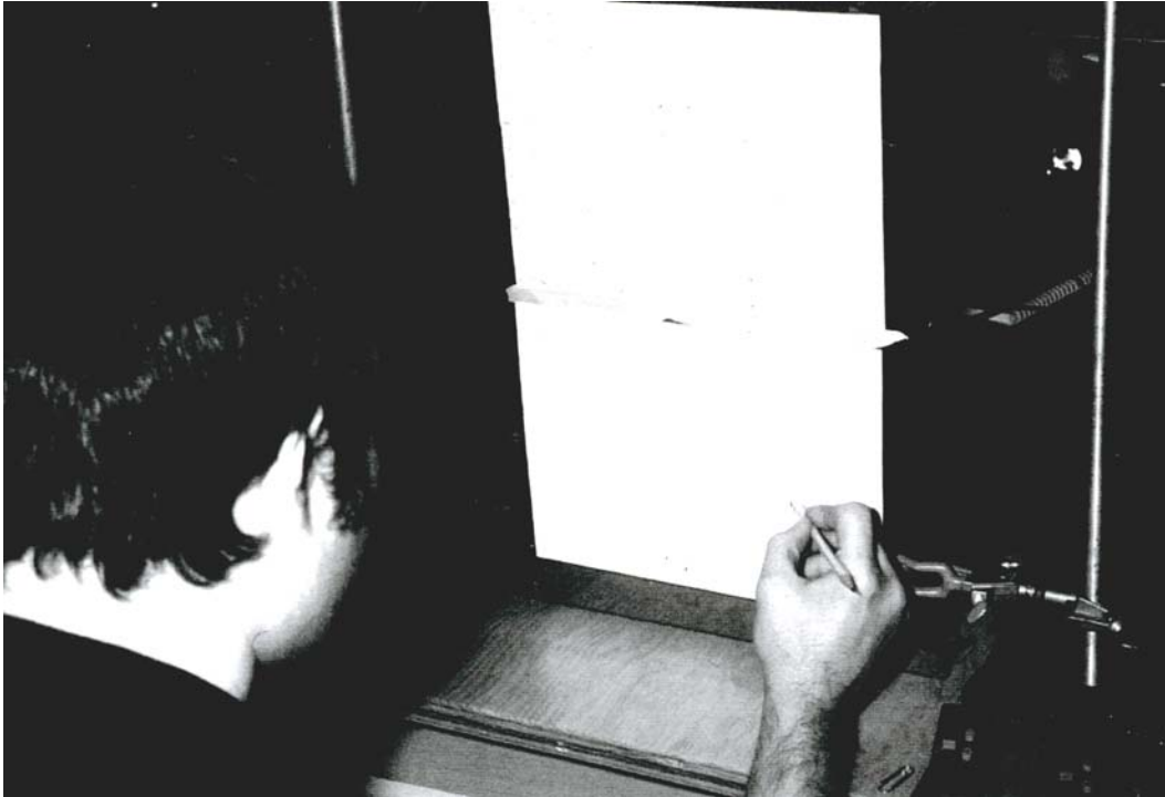
Fig. 6-13. Slides being scored in the laboratory using field notes. A 35-mm color slide of a field plot has been projected onto a piece of paper containing a grid of points. The grid is taped to a glass panel and the slide is projected from a position on the opposite side of the panel to eliminate shadowing.
